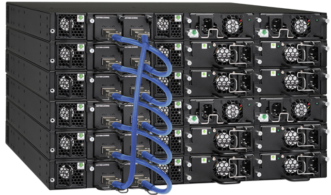
Figure 1: RUCKUS ICX switches can be stacked together using standard SFP+ or QSFP+ ports and optics to create a single logical device over distances up to 10 km.
