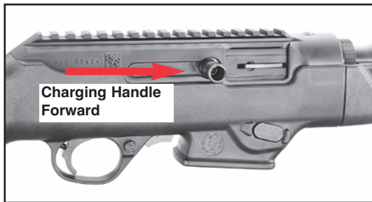
Figure 14. Location of Charging Handle for Disassembly
