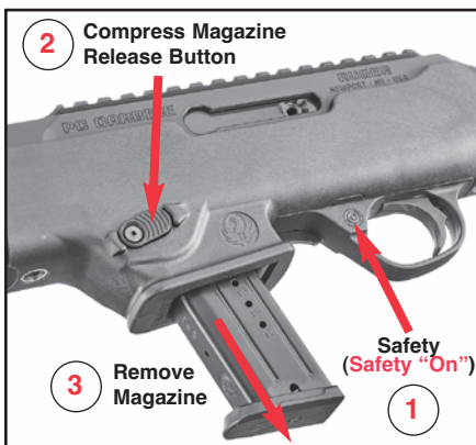
Figure 21. If the hammer is cocked, the safety should be “ON” when the magazine is being removed or inserted. When the magazine release button is pushed in, the magazine is released. Depress the button with your thumb and at the same time grasp the magazine and draw it downward out of the gun. REMEMBER to check to be sure the chamber is empty after removing the magazine!
