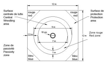
The central circle indicates the middle of the mat (1 m diameter). The inside part of the mat which is inside the red circle is the central surface of wrestling (7 m of diameter). The red strip (1 m width). The area in the protection area is 1.50 m width
