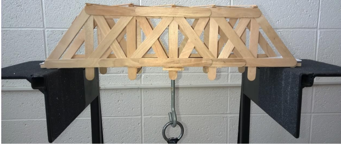
Figure 3: A bridge spanning the abutments of the test rig.
