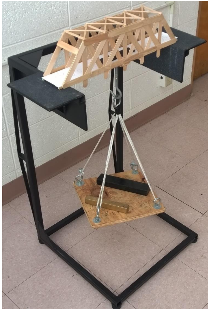
Figure 10: A bridge spanning the two test rig abutments with the loading equipment attached and carrying 2 lb and 5 lb weights.
