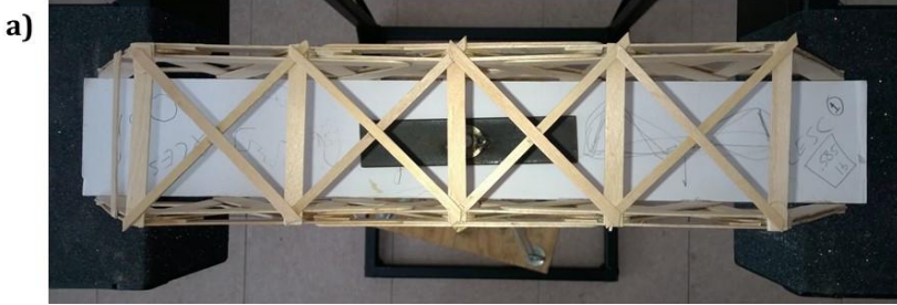
Figure 7: a) A top view of the load hanger attached to a bridge. b) A view down the span of a bridge with the load hanger attached.
