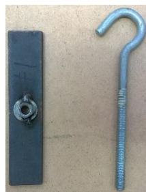
Figure 6: The steel plate and hanger bolt that make up the loading hanger assembly.
