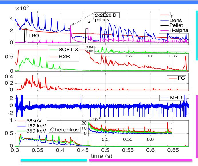
Instability with high REs energies: no MHD signs, sharp n<sub>e</sub> spikes with density peaked at the magnetic axis (quite peaked), spikes on FC, Cherenkov and soft-x. [new type of instability?]
