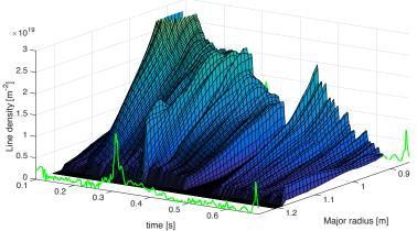
Interferometer: the large oscillations after 0.5s are larger toward the low field side and seem to be in advance with respect to high field side.
