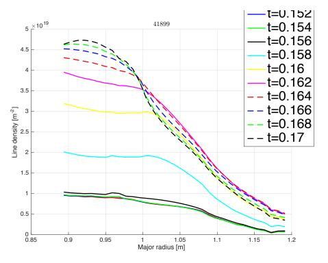
Density profiles Vs major radius at different time for the first small pellet in **the flat-top discharge**.
