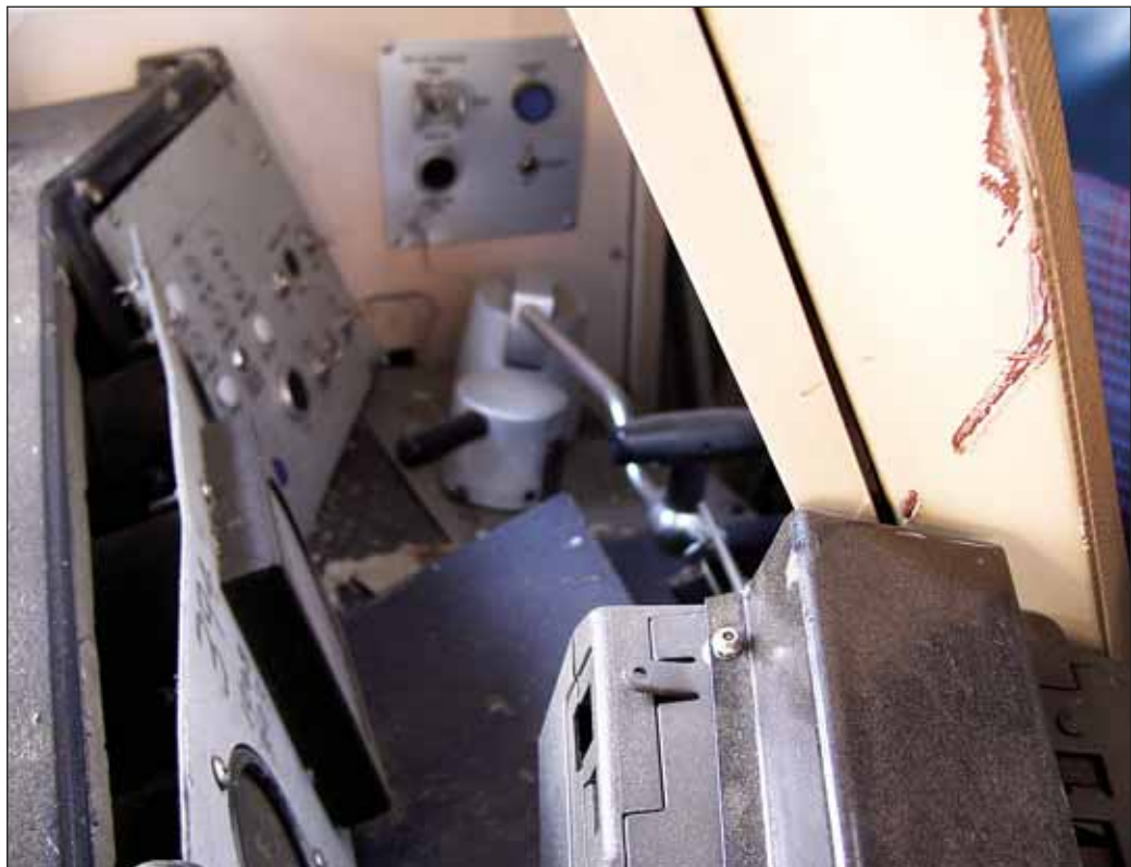
FIGURE 7: Damage to drivers cabin, car 394
