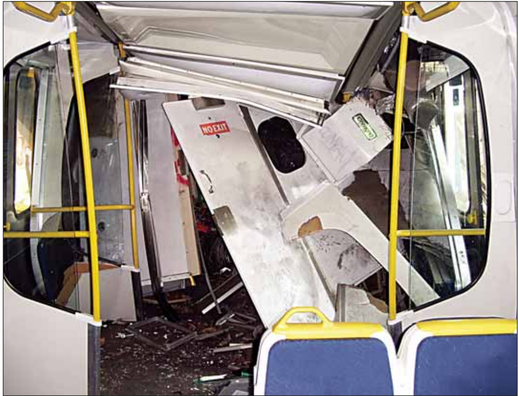
FIGURE 8: Damage to passenger vestibule car 394
