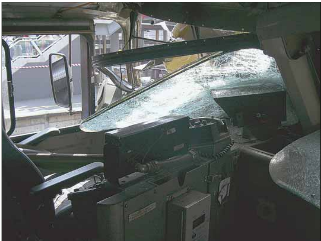
FIGURE 9: Damage to driver's cabin, N463
