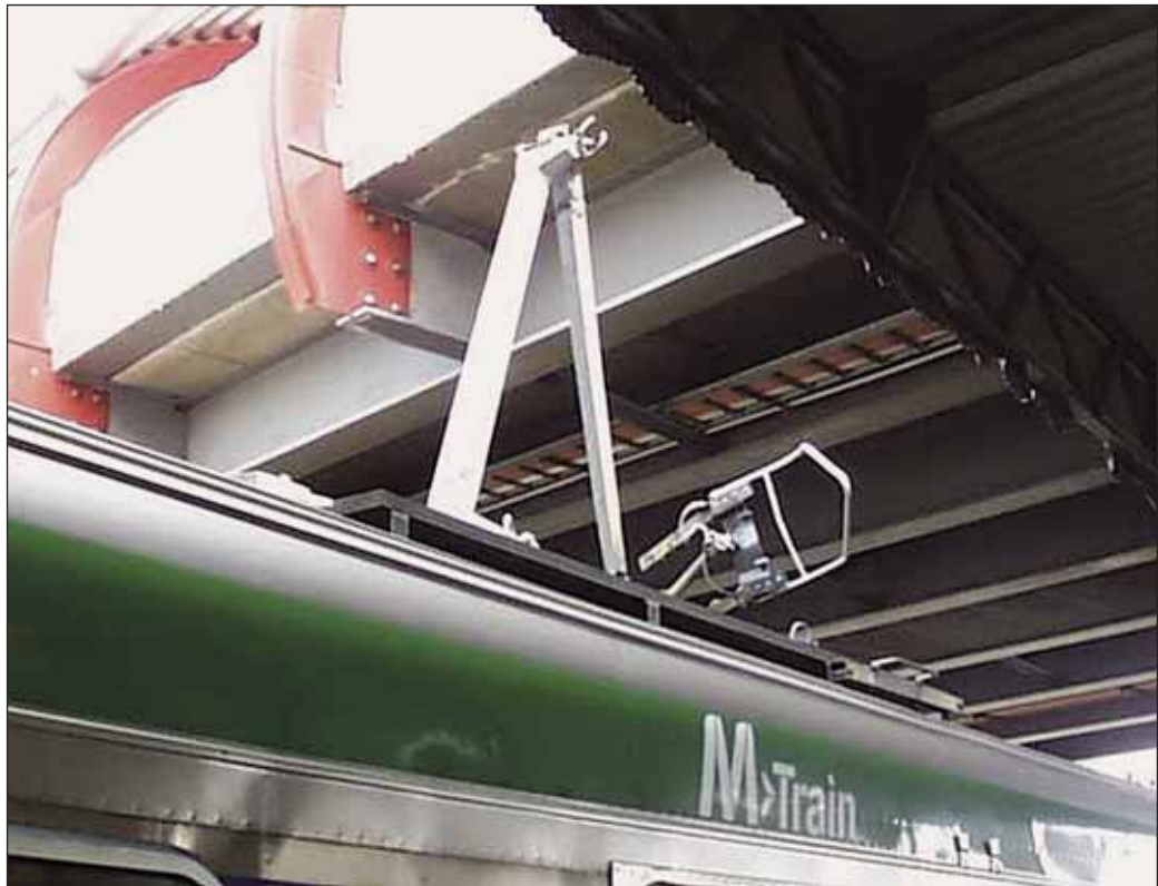
FIGURE 10: Damaged fully extended pantograph
