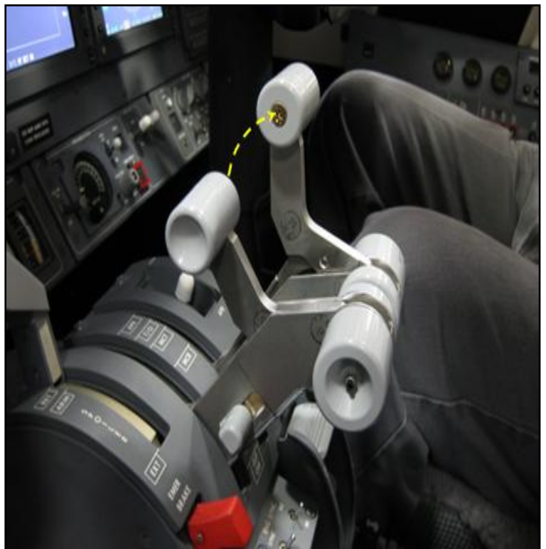
Figure 2. Captain's side view of Learjet 60 thrust levers (at idle) and thrust reverser (piggyback) levers. To illustrate lever movement, one thrust reverser lever is in the stowed position, and the other is lifted to command reverse thrust (arrow shows direction lever moves when lifted from the stowed position).
