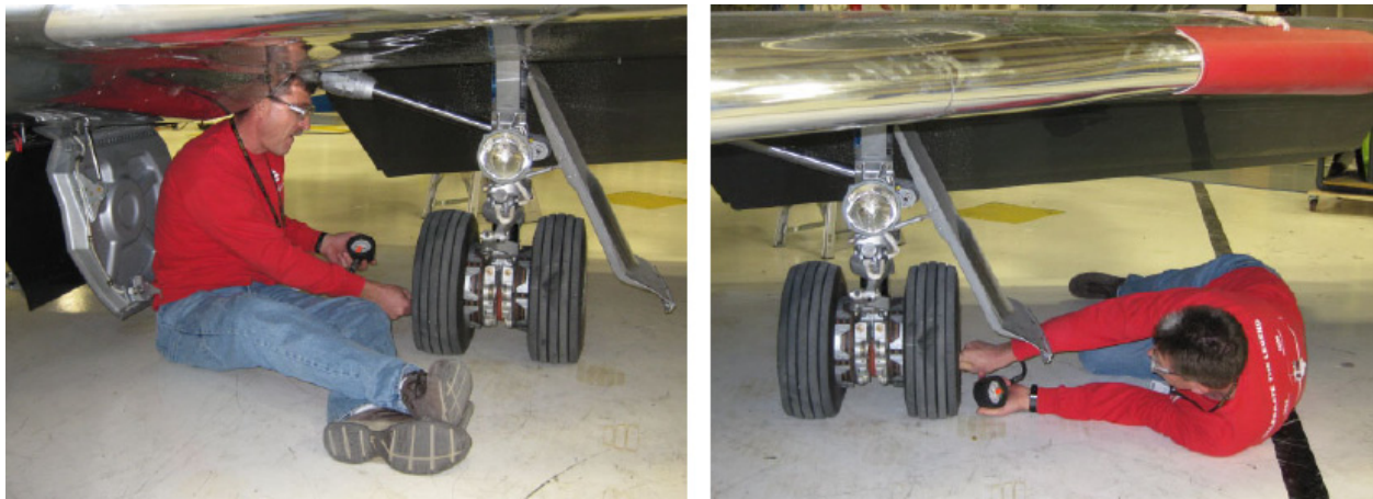
Figure 1. Learjet factory technician checking inboard tire pressure (left image) and outboard tire pressure (right image).
