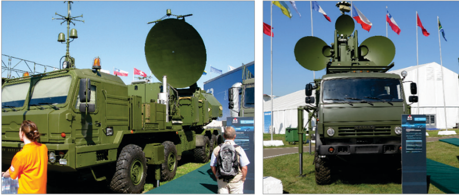
Figure 17 & 18: Jamming system Krasukha-2O and Krasukha-4S . Source: The Swedish Defence Material Administration.
