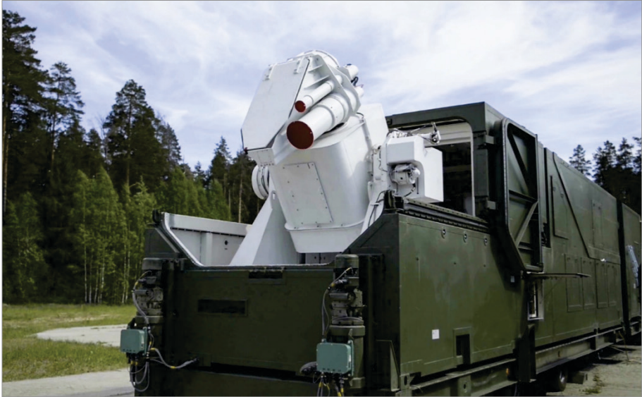
Figure 30: Russian laser weapon Peresvet . Source: TT Nyhetsbyrån.
