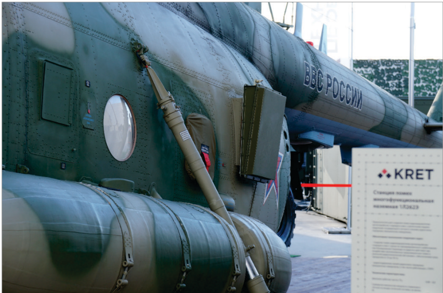
Figure 23: Antenna of the Rychag-AV helicopter EW system. Source: The Swedish Defence Material Administration.
