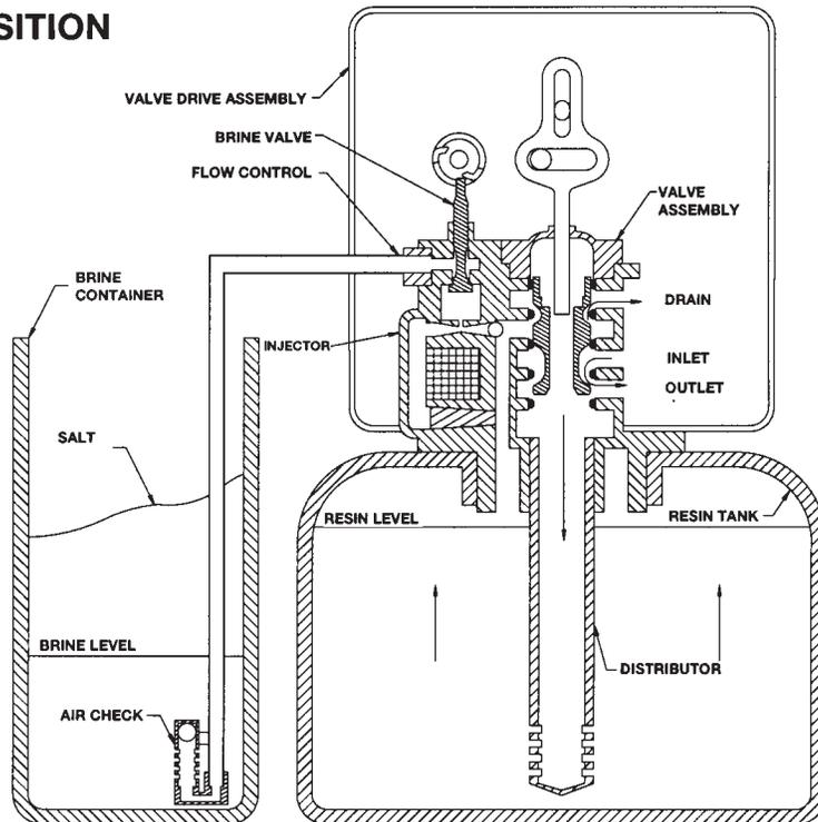
Hard water enters unit at valve inlet - flows around piston - down center tube - thru bottom distributor and up thru the mineral - around the piston and out the drain line.
