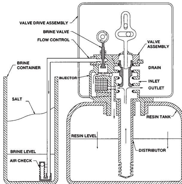
Hard water enters unit at valve inlet and flows around the piston down thru the mineral. Conditioned water flows up thru the center tube - flows thru the injector housing - thru the brine valve to fill the brine tank.
