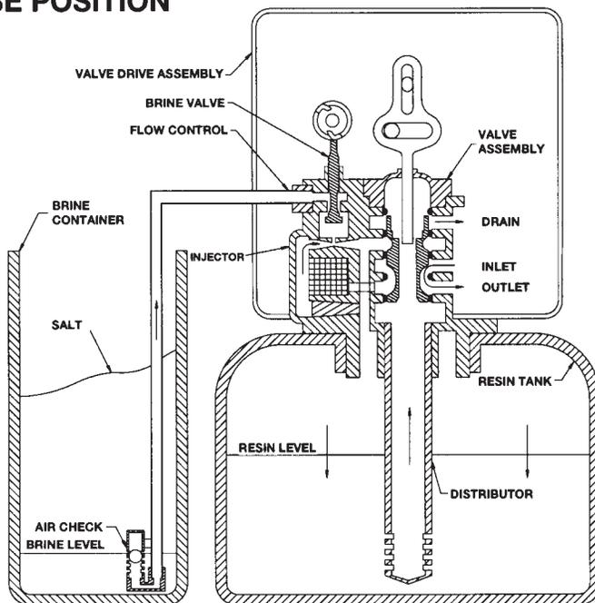
**Brine.** Hard water enters unit at valve inlet - flows into injector housing and thru nozzle and throat to draw brine from the brine tank - brine flows down thru mineral and enters the center tube thru bottom distributor and out thru the drain line.
