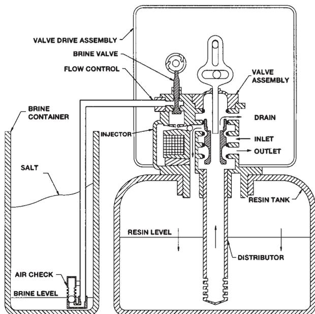
Hard water flows from inlet around the piston down thru the mineral into bottom distributor and up thru center tube - thru piston and out thru the drain line.
