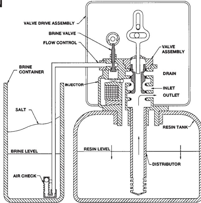
Hard water enters unit at valve inlet and flows around the piston down thru the mineral in the mineral tank. Conditioned water enters center tube thru the bottom distributor - then flows up thru the center tube and to the outlet of the valve.
