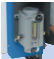
Centralized oiling system
