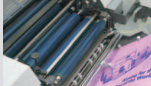
Crestline continuous dampening system
