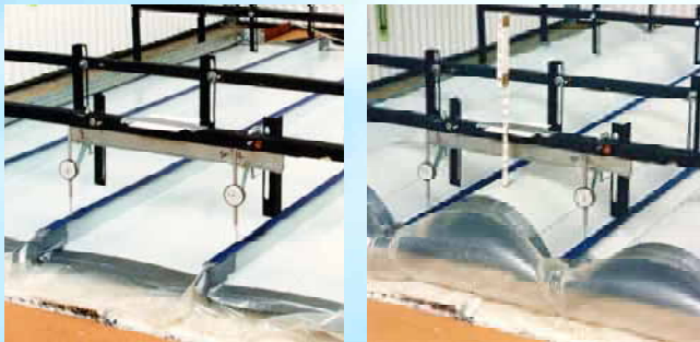
SRS panels have been tested to achieve allowable uplift loads in excess of 180 psf [8.62 kPa] in accordance with the ASTM E 1592 test specification.
