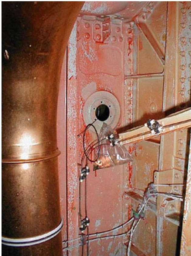
Figure 2 - Purge door opening. Fuel and retaining screws inside plastic bag. Purge door is hanging on lanyard inside the fuel tank. The O-ring seal was removed from the purge door by maintenance staff following the incident.
