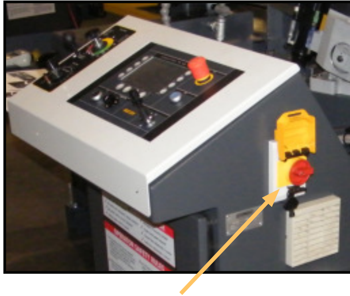
Machine Disconnect Switch
