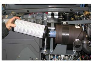
Replace the safety filter element after the primary has been changed three times. Do not remove the safety filter element from the housing unless it is restricting air flow.
