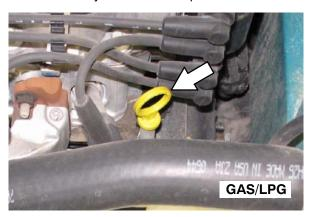
Gas/LPG engines: Fill the engine with oil until the oil is between the indicator marks on the dipstick. DO NOT fill past the top indicator mark. The engine oil capacity is 3.5 L (3.7 qt) with oil filter.
