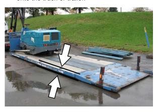
4. To winch the machine onto the truck or trailer, attach the winching chains to the holes in the right and left lower corners in front of the machine.
