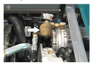
Disassemble the fuel lock off valve to access the LPG fuel filter.
