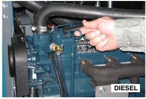
Diesel engines: Fill the engine with oil until the oil is between the indicator marks on the dipstick. DO NOT fill past the top indicator mark. The engine oil capacity is 6 L (6.35 qt) with oil filter.
