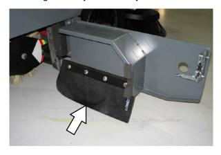
NOTE: The brush door skirts have slotted holes to allow for a ground clearance adjustment. The door must be closed for proper adjustment.
