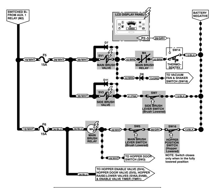
Thermo-Sentry switch (SW14) is shown in the normal NON-activated position (13/BLK connected to 52/BRN). The switch is activated (13/BLK connected to 28/GRY) when the Hopper air temperature exceeds 71°C (160°F). The Hopper Fire indicator on the LCD panel will also illuminate when this switch is activated. When the temperature falls below 60°C (140°F), the switch will return to the NON-activated position, and the indicator light will turn OFF.
