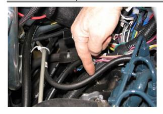
The rubber fuel lines can become worn-out whether the engine has been used much or not. Replace the fuel lines and clamp bands every two years.
