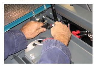
3. Remove the filter shaker assembly from the filter housing.
