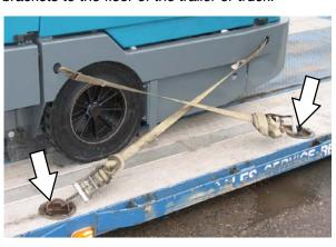
FOR SAFETY: When unloading machine off truck or trailer, use winch. Do not drive the machine off the truck or trailer unless the loading surface is horizontal AND 380 mm (15 in) or less from the ground.
