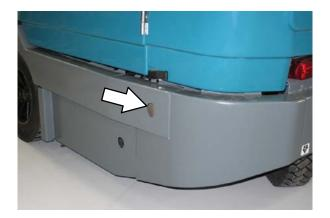
Route the tie-downs to the opposite ends of the machine and hook them to the brackets on the floor of the trailer or truck. Tighten the tie-down straps.
