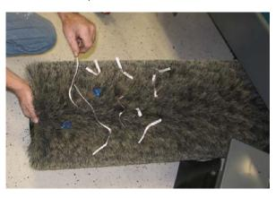
Check the main brush pattern and rotate the brush end-for-end after every 50 hours of operation, for maximum brush life and best sweeping performance. Refer to REPLACING OR ROTATING THE MAIN BRUSH.
