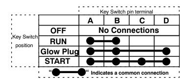
$oxed{oxed{i}}$  Common connections in various switch positions should be less than 1  $\Omega$
