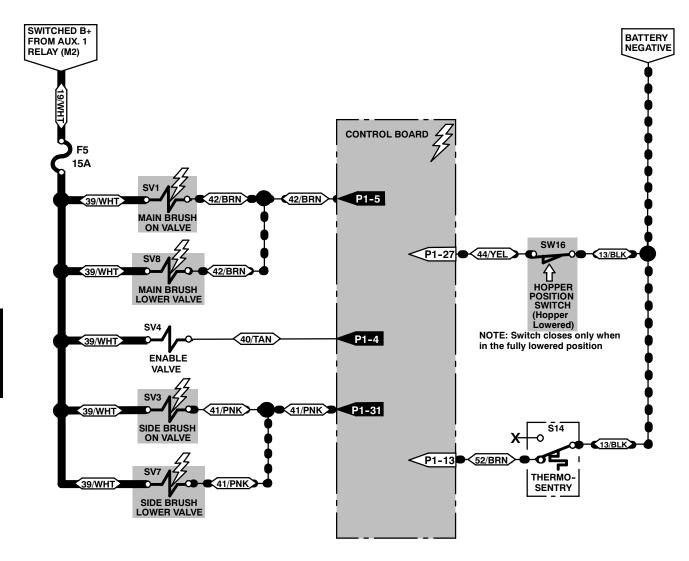
Thermo-Sentry switch (S14) is shown in the normal NON-activated position (13/BLK connected to 52/BRN). The switch is activated (13/BLK connected to 28/GRY) when the Hopper air temperature exceeds 71°C (160°F). The Hopper Fire indicator on the control panel will also illuminate when this switch is activated. When the temperature falls below 60°C (140°F), the switch will return to the NON-activated position, and the indicator light will turn OFF.
