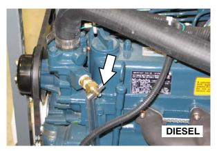
Check the radiator hoses and clamps after every 200 hours of operation. Tighten loose clamps. Replace damaged hoses and clamps.
