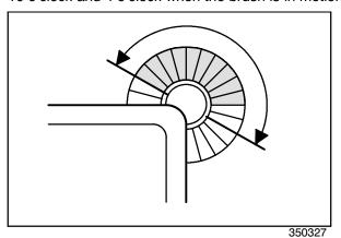
**S30:** Turn the *side brush adjustment knob* counterclockwise to increase the brush pattern and clockwise to decrease the brush pattern.
