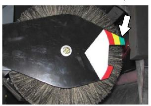
2. Loosen the main brush adjustment knob and slide the pointer so it matches the color band on the brush idler plate. Retighten the knob.
