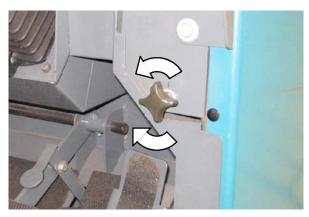
**S30XP and S30X4:** Tighten the *side brush adjustment knob* into the side brush bracket to increase the brush pattern and loosen the knob to decrease the brush pattern.
