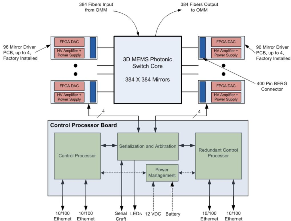
**Figure 3: MSM320 block diagram**
