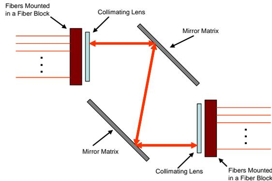
**Figure 2: Light path within the MSM320**
