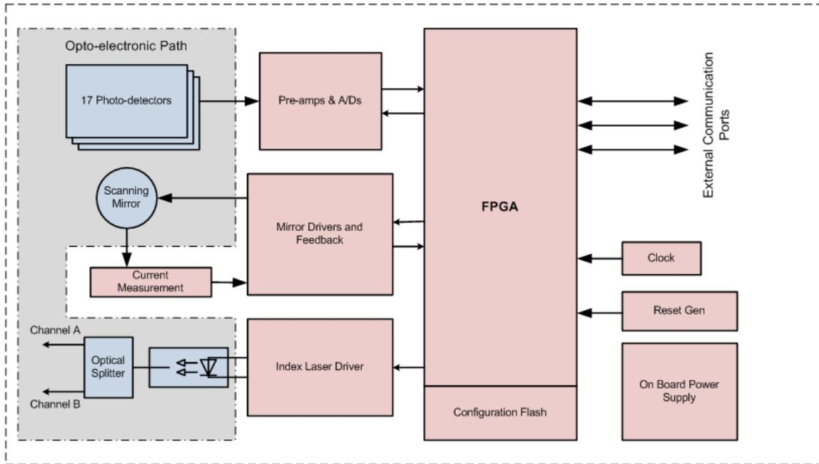
**Figure 5: OMM block diagram**
