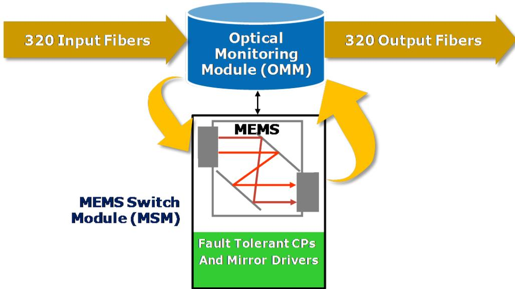
**Figure 1: CALIENT S320 Photonic Switch Architecture**
