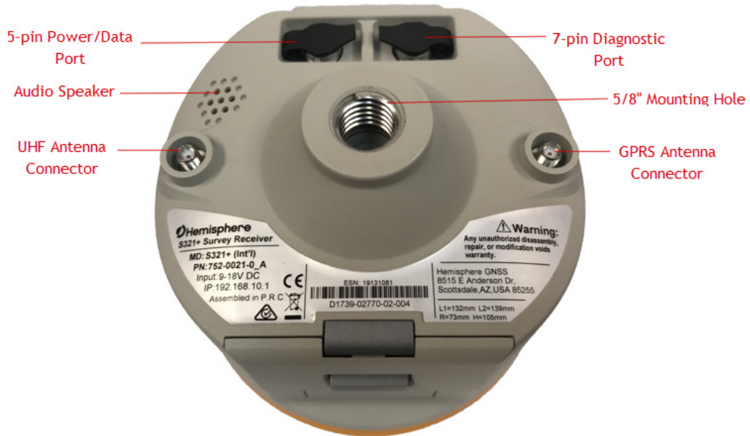
Figure 2-1: S321+ ports and connectors
