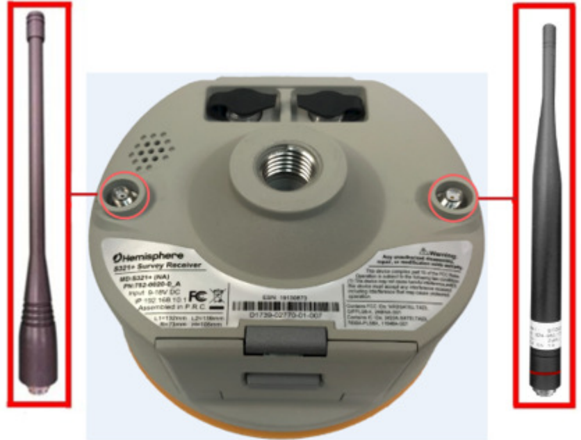
Figure 2-3: Installing UHF and GSM antennas
