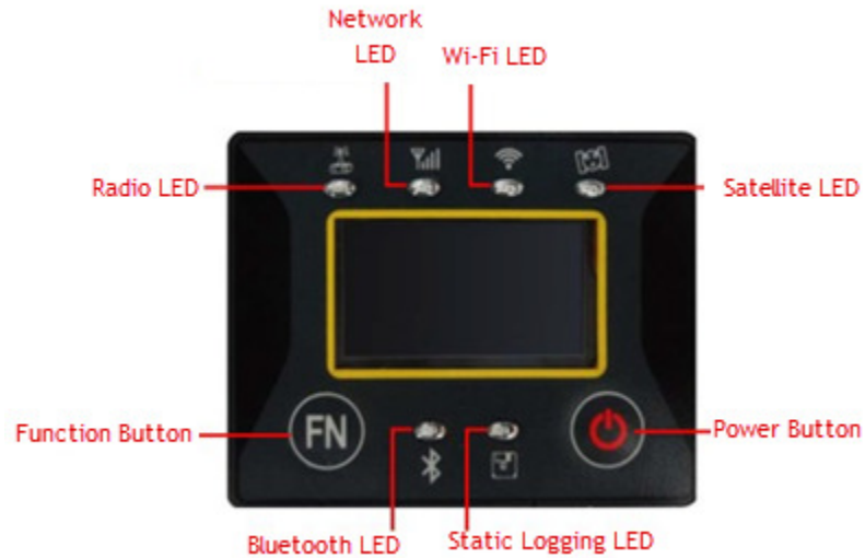
Figure 3-1: Control Panel and display
