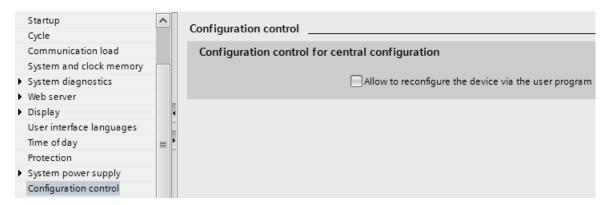
Create a control data record (in a data block, for example) according to the current configuration based on the sample described below for the control data record. The control data record has the number 196.
