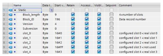
In the startup OB, call the extended WRREC (Write data record) instruction and transfer the created control data record.
