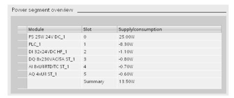
Figure 4-7 Example of a power balance calculation with STEP 7
