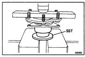
(d) Using SST and a press, install the bearing. SST 09316–60010 (09316–00040)
