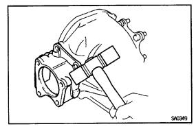
(b) Using a plastic–faced hammer, tap on the clutch case to remove it.
