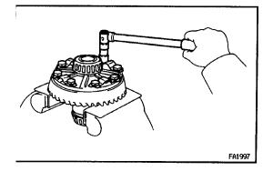
(c) Remove the 10 bolts and 5 lock plates.
