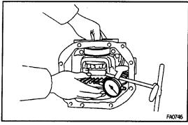
(c) Hold the side bearing boss on the teeth surface of the ring gear and measure the backlash.
