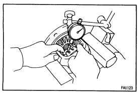
(d) Measure the side gear backlash while holding 1 pinion gear toward the differential case.
