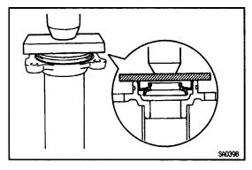
(b) With the oil seal lip facing upward, use press and plate to press in a new oil seal until its end is flush with the surface of the tube.
