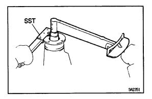
If the preload is greater than the specification, replace the spacer.
