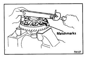
HINT: Align the matchmarks on the ring gear and differential case.
