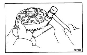
(d) Using a plastic–faced hammer, tap on the ring gear to separate it from the differential case.
