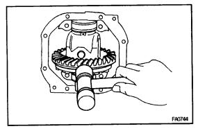
Tap on the ring gear with a plastic–faced hammer so that the washer fit to bearing.
