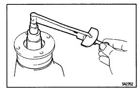
(f) Using a torque wrench, measure the preload.
