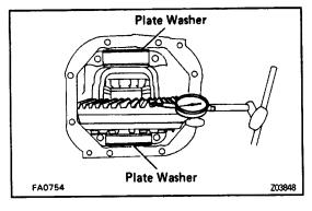
(k) If the backlash is not within specification, adjust b) either increasing or decreasing the number of washer: on both sides by an equal amount.
