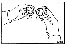
(b) Install the proper thrust washers on the side gears. HINT: Using the table below, select thrust washers which will ensure that the backlash is within specifications. Washer thickness
