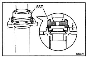
(c) Using SST, press in the oil seal. SST 09554–14010
