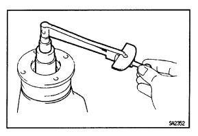
(b) Using the backlash as a reference, install a new washer of 0.06-0.09~mm~(0.0024-0.0035~in.)
