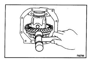
(b) Tap on the ring gear with a plastic–faced hammer so that the washer fit to bearing.
