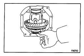
(d) Select a ring gear back side plate washer, using the backlash as reference. (See page SA-73)
