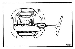
(j) Using a dial indicator, measure the ring gear backlash **Backlash**:
