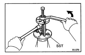
(c) Using SST, remove the companion flange. SST 09950 – 30010
