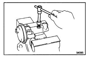
(b) Coat the threads of screw plug with FIPG.
