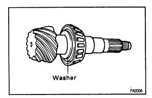
If the teeth are not contacting properly, use the following chart to select a proper washer for correction.
