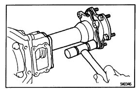
(b) Using a plastic–faced hammer, tap on the tube to remove it.
