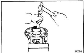
(c) Using a brass bar and hammer, drive out the needle labearings.
