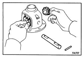
(c) Install the side gears, pinion gears, pinion gear thrust washers and pinion shaft in the differential case.HINT: Align the holes of the differential case and pinion shaft.
