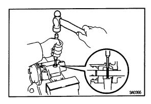
(b) Using a pin punch and hammer, drive out the pin through the hole of clutch case cover.
