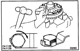
(g) Using a hammer and drift punch, stake the lock in plates
