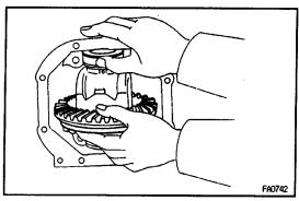
(e) Select a ring gear teeth side plate washer with a thickness which eliminates any clearance between the outer race and case.
