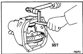
(c) Using SST, remove the 2 side bearing plate washers. SST 09504–22011
