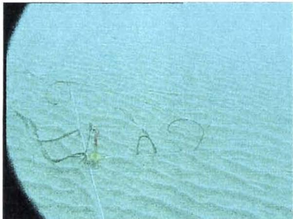
**Figure 4** *Picture of bottom ripple structure with buried hydrophone array.*
