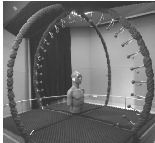
(Figure 15 - Example of HRTF measurement based on a dummy head - Zhong and Xie, 2014)
