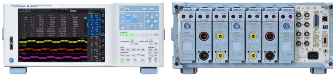
Figure 2 – Multi-phase power analyzer
