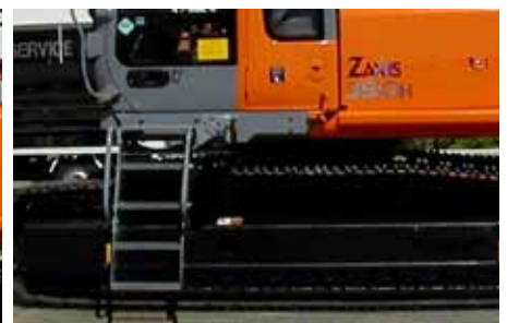
RotorStep L in the extended position
