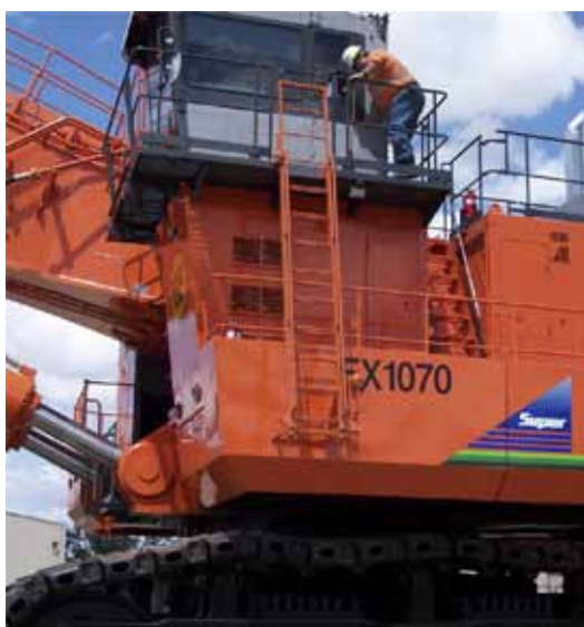
Model EF Ladder shown fitted to excavator in the up and down positions
