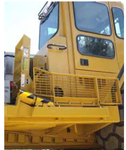
RotorStep S Ladder shown fitted to a Cat 657 scraper
