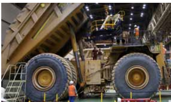
Trilift® Cat 797 Transmission Hoist removing transmission
