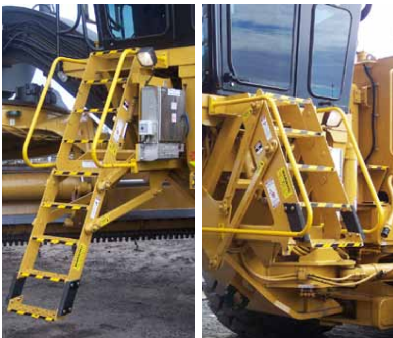
Cat 24H Access System shown lowered and retracted
