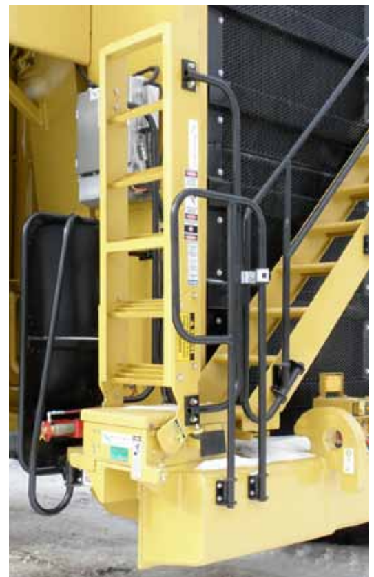
Model RTV-LNS Ladder shown fitted to truck
