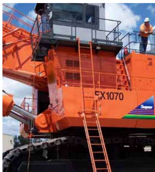
Model EF Ladder shown fitted to excavator in the up and down positions
