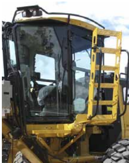
RotorStep GM Ladder shown fitted to a Cat 16M Grader
