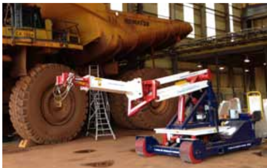
Trilift® Variable Work Table with Multijig and Cylinder Handler
