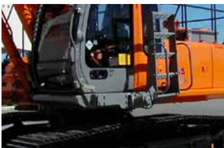
RotorStep L in the retracted position
