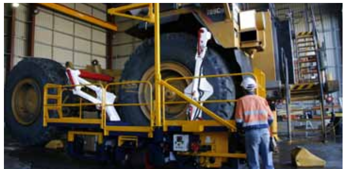
Trilift® TH15000 Workshop Tyre Handler removing Cat 789C tyre
