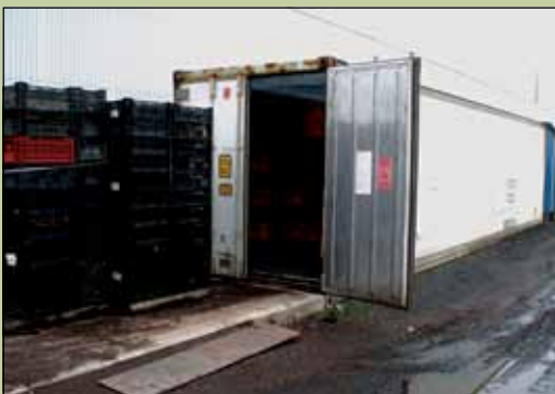
Fig. 7.2.1.e — Insulated shipping container modified as a steam chamber for pasteurizing used containers and propagation flats.
