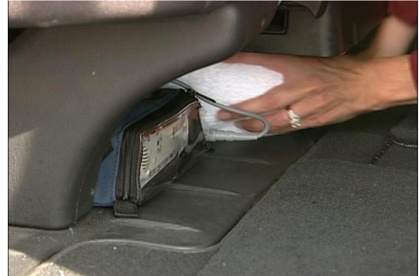
Apnea monitor being wedged under vehicle seat with towel roll
