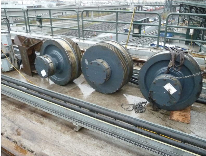
Interim Wheel Assemblies Ready for Installation
