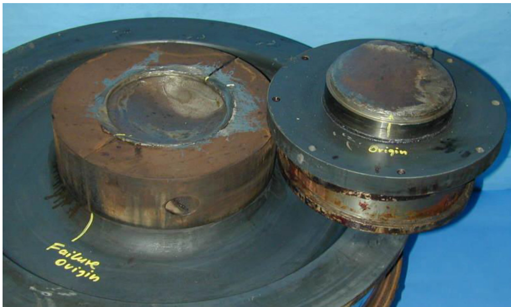
Initial Axle Failure at Locking Collar Groove
