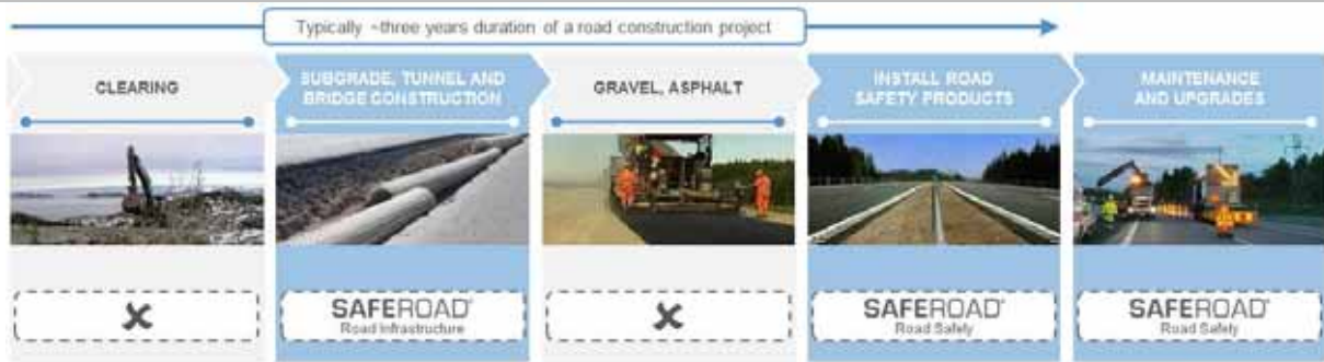
Figure 7.1.3: Phases of a road construction project
