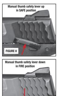
The trigger of the M&P<sup>o</sup> 9 SHIELD<sup>™</sup> EZ<sup>o</sup> with a manual thumb safety can still be depressed (without firing the pistol) when the manual thumb safety lever is in the SAFE position.
