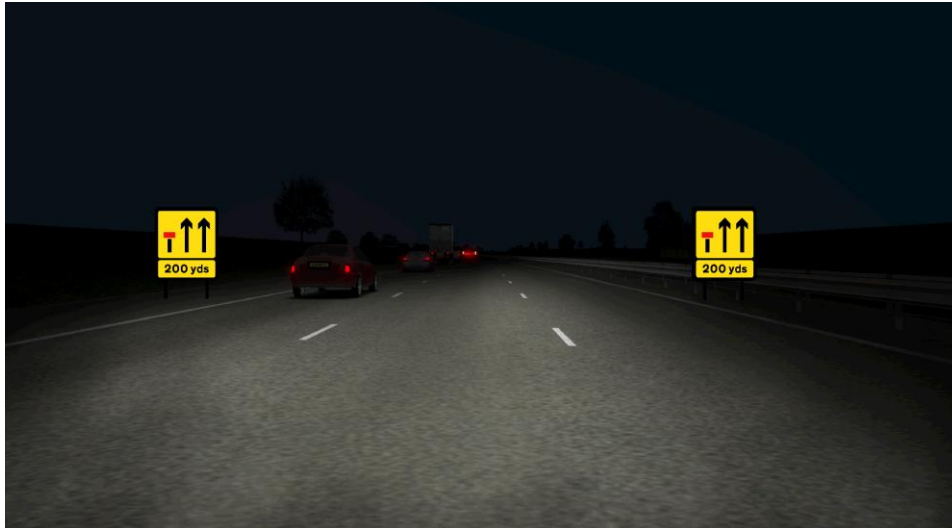
Figure 14. Example of display screen showing a pair of wicket signs warning drivers of a lane 1 closure ahead at 200 yards
