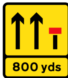
Figure 11. Wickets sign with supplementary distance plate sign showing an offside lane closure at 800 yards ahead
