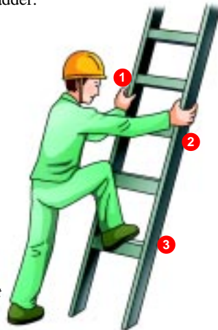
Face the ladder and maintain a three-point contact when moving up and down.
