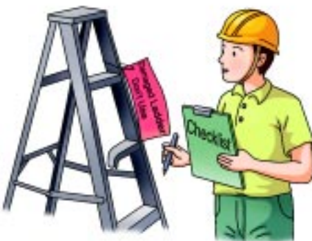
Label the damaged ladder.
