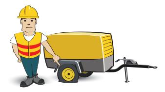
Make sure all wheel bolts, lugs, and nuts are tightened to Atlas Copco instructions. Do not change tire sizes or types.
