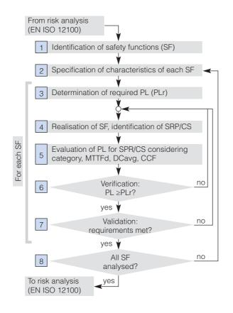
$\begin{array}{l} SF = safety \mbox{ function} \\ PL = \mbox{ performance level} \\ PLr = \mbox{ required performance level} \\ SRP/CS = safety-related \mbox{ parts of control systems} \\ MTTF_d = \mbox{ mean time of dangerous failure} \\ DCavg = \mbox{ average diagnostic coverage} \\ CCF = \mbox{ common cause failure} \end{array}$
