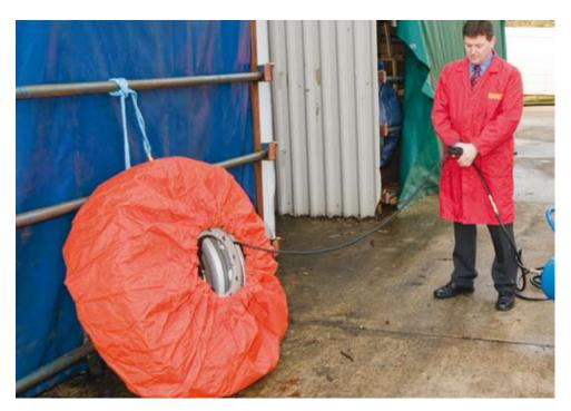
Figure 5 A bag-type restraint
