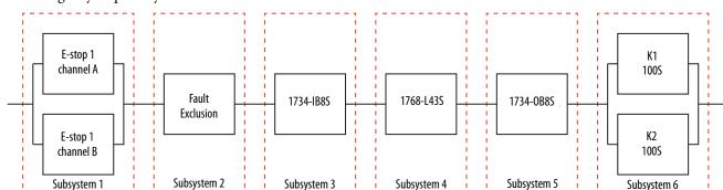
The emergency stop safety function can be modeled as follows.
