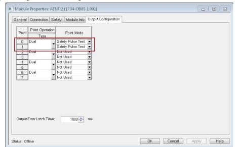
6. Click Output Configuration and configure the module as shown.
