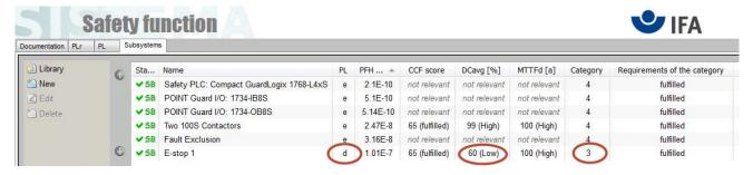
Calculations are based on one operation of the E-stop per month, with 12 operations per year. Because there are three E-stops in this safety function, there are 36 operations of the contactors per year.
