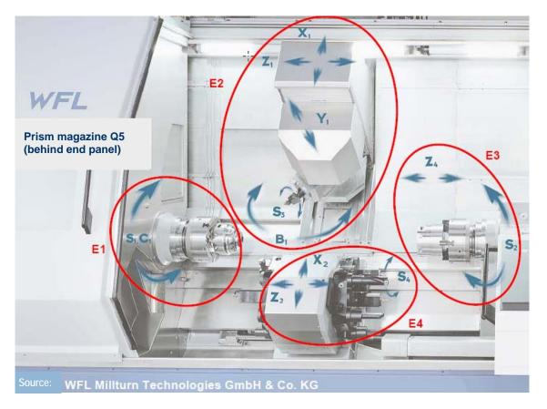
Analysis of the four discrete hazards of machine parts thus yields four safety functions, SF1 to SF4, which result in a risk reduction for E1 to E4:
