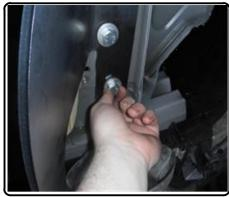
6. Torque 1/2" hardware to 110 lb-ft and M12 hardware to 79 lb-ft.
