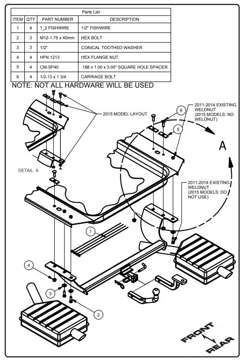
1. Locate and remove (2) exhaust isolators near muffler on driver and passenger side of vehicle. Save bolts for reinstallation.
