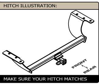
PERIODICALLY CHECK THIS RECEIVER HITCH TO ENSURE ALL FASTENERS ARE TIGHT AND ALL STRUCTURAL COMPONENTS ARE SOUND
