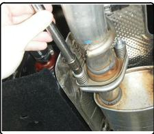
8. Raise exhaust back into position and reattach (2) exhaust isolators. Reinstall (4) hangers removed in Step 1.
