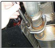
4. Fishwire 1/2" carriage bolts and CM-SP40 spacers through access hole on driver and passenger side frame rail. Pull hardware through existing holes (2 on passenger side and 1 on driver side) (2015 Models: fishwire 3 carriage bolts on passenger side).
