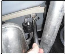
2. Locate and remove (2) rubber isolators from exhaust pipe.
