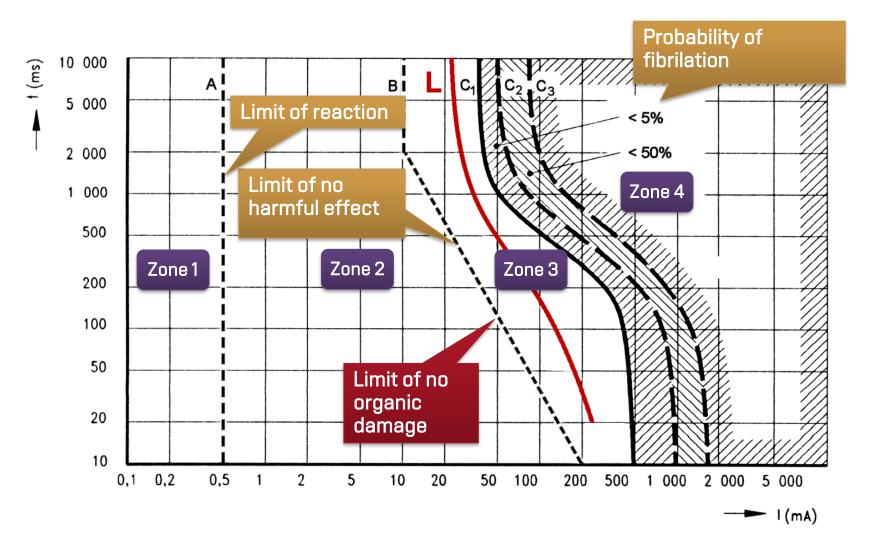
This diagram is valid for AC 15-100 Hz , way of current left hand to both legs
