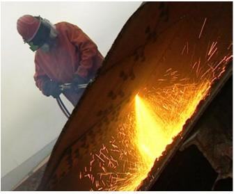
Figure 2 Cutting up scrap
