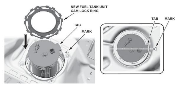
11. Lock the fuel tank unit cam lock ring.
