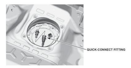
Connect the fuel tank unit connector.
