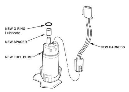
9.2. Install the fuel pump to the fuel filter.
