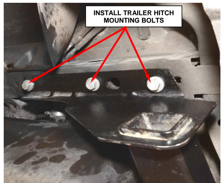
Figure 10 – Install Mounting Bolts (left side shown)
