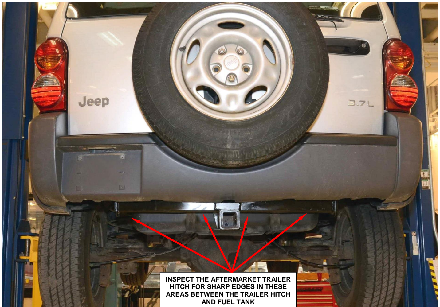
Figure 3 – Inspect Aftermarket Trailer Hitch
