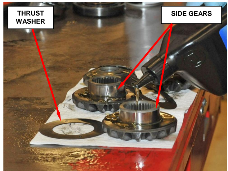
Figure 44 – Lubricate Side Gears and Thrust Washers
