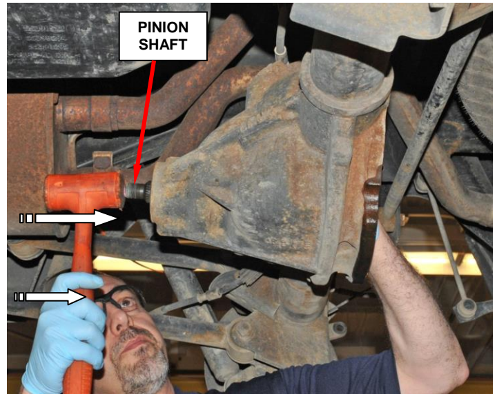
Figure 12 – Pinion Gear Removal
