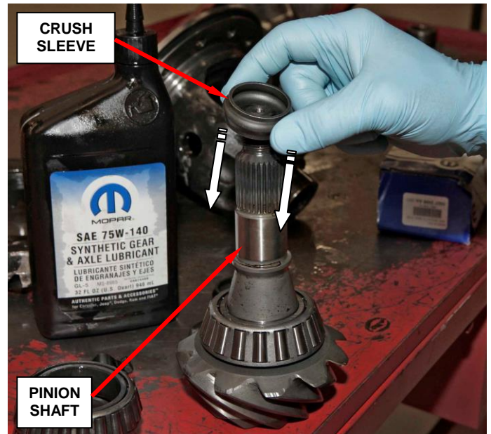
Figure 26 – Install New Crush Sleeve
