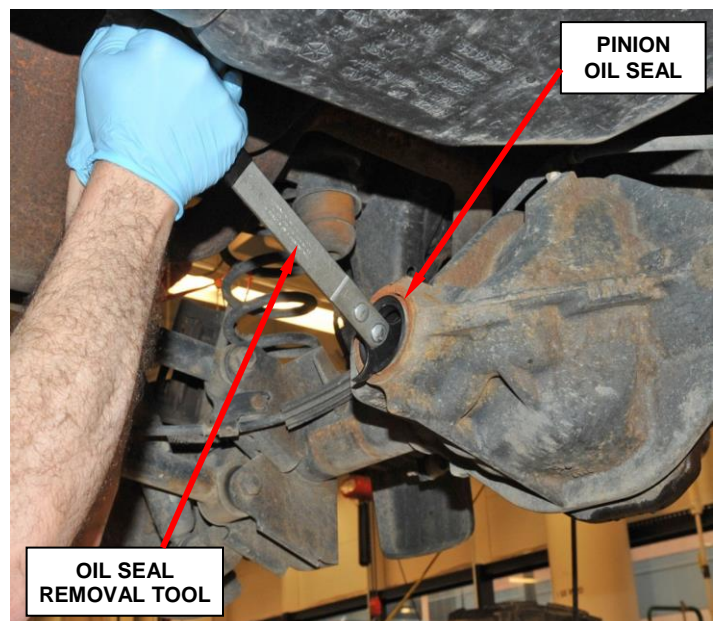
Figure 13 – Pinion Oil Seal Removal
