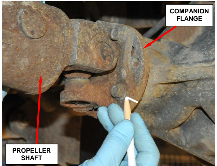
Figure 1 – Mark Propeller Shaft-to-Companion Flange Orientation
