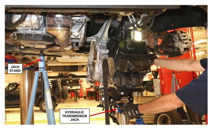
Figure 31 - Lower Transaxle from Vehicle
