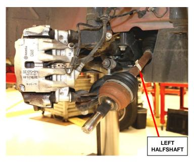
Figure 25 - Left Halfshaft
