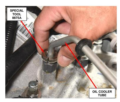
Figure 3 - Oil Cooler Tubes
