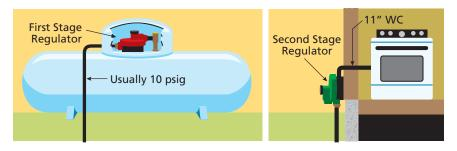
**FIGURE 2-5 LPG tank regulator system.** NOTE: WC = water column.
