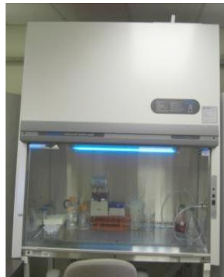
Example of biosafety cabinet with germicidal lamp
