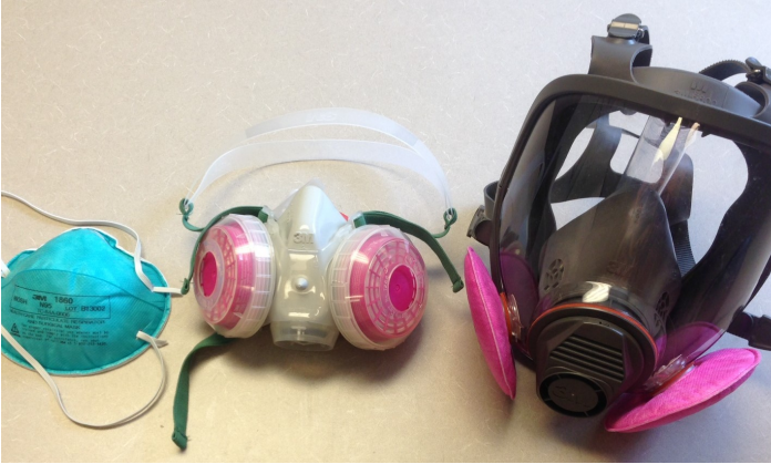
Figure 9. Disposable filtering facepiece (left), reusable half-mask respirator with particulate filters (middle), and reusable full face respirator with particulate filters (right).
