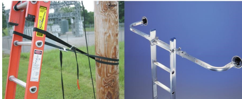
Figure 11. Ladder straps (left) can help reduce kick-outs and a stabilizer (right) keeps a ladder away from a structure.
