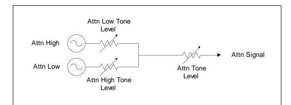
Figure 4-3. DSP-based ATTN signal level adjustments. The Data tone is similar. Individual tones can be adjusted for pre-emphasis.
