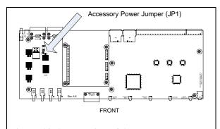
Figure 13-1. Location of Accessory Power Enable Jumper JP1.
