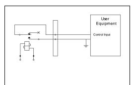
Figure 4-7. As a contact closure for a control input.
