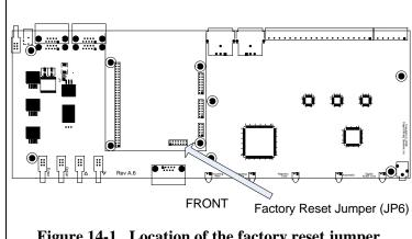
Figure 14-1. Location of the factory reset jumper.
