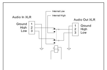
Figure 4-2. Main Audio XLRs, one channel. Left and right are identical.
