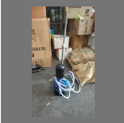
Cement Grouting Pump 140 Psi
