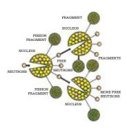
Nuclear fission (splitting) occurs when the nucleus of an atom of U235 Uranium is bombarded with neutrons from another source. The nucleus splits into two smaller fragments and at the same time releases additional neutrons. Some of these additional neutrons will split other U235 nuclei which in turn will release still more neutrons. This continuous splitting is a chain reaction. One product of a chain reaction is heat produced by the fragments being scattered at high speed.
