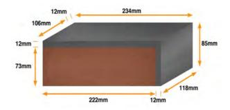
The format length, i.e. 234mm is the spacing of stretcher perpends. The format width, i.e.118mm is the spacing of header perpends. The format height, i.e. 85mm is the coursing height. It should also be noted that the actual length of a brickwork panel is less by one 12mm joint than the overall distance between format lines - Figure 6.2
