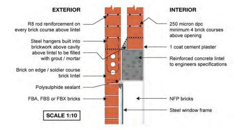
Note: This detail is suitable for a multi-story building where there is no protection from rain to the area above the window
