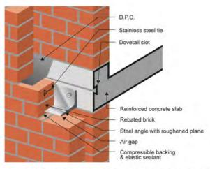
Steel angle / bricks arrangement showing positioning of ties and damp proof course.
