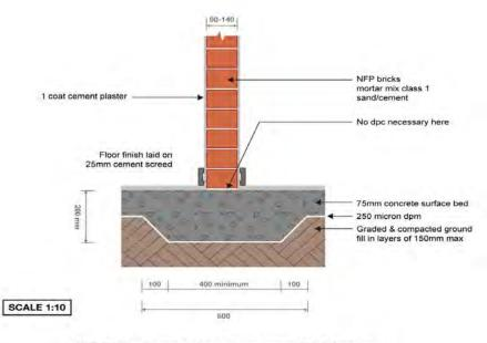
NOTE: This detail is suitable for areas where ground fill is 300 maximum and where internal walls are kept to a minimum height
