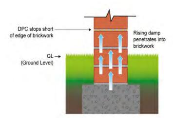
Figure 8.7: Not taking DPC right through mortar joint
