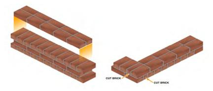
*Note:* A wall comprising of two brick leaves is known as a full brick wall, and a wall with only one leaf is a half brick wall.
