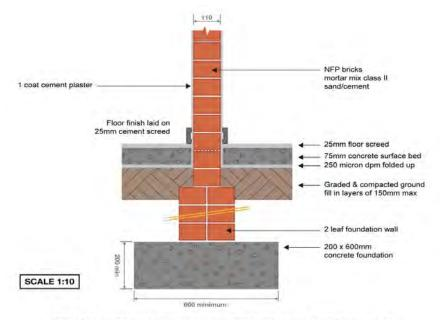
NOTE: This detail is suitable where internal foundation wall exceeds 75 - 1000mm in height
