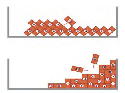
A frequently encountered form of flexible paving is 'butt jointing'. Butt jointed paving invariably has less than the necessary joint width and may cause the surface to act locally in a semi-rigid manner. Direct contact between adjacent fired clay pavers is a highly undesirable practice for it can lead to chipping of adjacent units under load. It is best to avoid infill pieces less than one third of a paver size by planning the pattern in advance.
