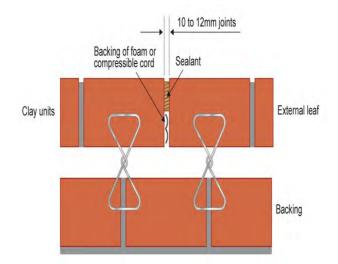
Figure 9.1: Metal Wall Ties in Composite Walling
