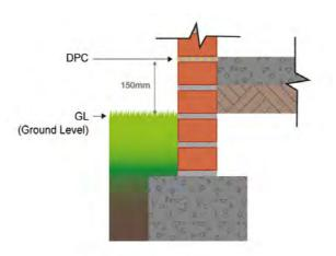
Various materials may be used for DPC, the most popular being black polyethylene sheeting which can be obtained in rolls. It provides a complete barrier against moisture penetration and is easy to store, handle and lay.
