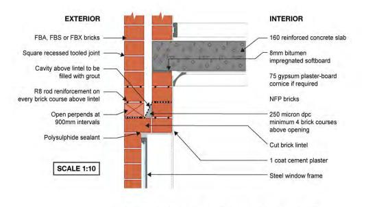
Note: This detail is suitable for a multi-story building where there is no protection from rain to the area above the window
