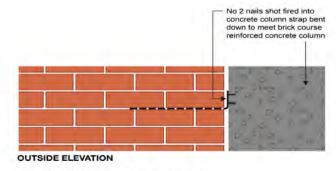
Note: Steel straps are to be built into mortar bed
