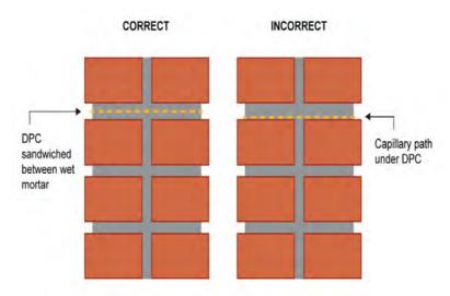
Figure 8.8: The sandwiching of DPC between wet mortar layers
