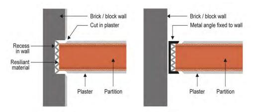
Figure 9.5: Plan view of Edge Isolation of Partitions
