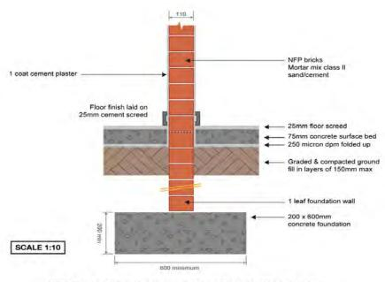
NOTE: This detail is suitable where internal foundation wall is 300mm in height
