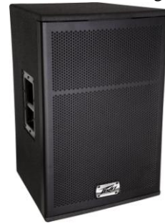
PEAVEY EU 115 Mid-Range Freq Rng 65Hz-18kHz Peak 1800W,125dB, 89x50deg cvg pattern
