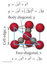
Starting in the lower right-hand corner of the unit cell, the distance from the center of the oxygen ion at the corner of the unit cell to the center of the oxygen at the body center of the unit cell is  $r(O^{2-}) + 2r(C^{u+}) + r(O^{2-}) = 2r(O^{2-}) + 2r(C^{u+})$ . Twice this distance is equal to the body diagonal, *y*.
